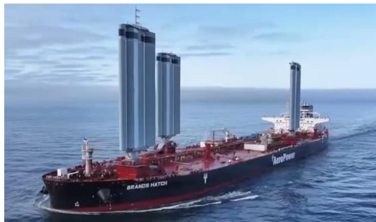
Wind-assisted propulsion system design as a whole with the hull
