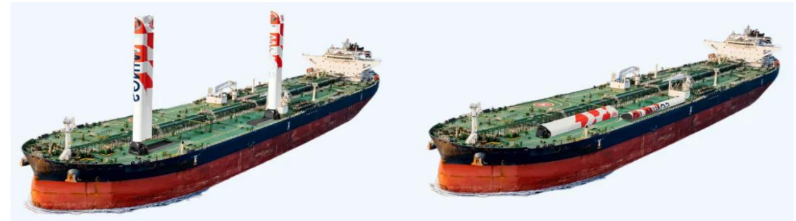
Wind-assisted propulsion system, modular design separated from hull design
