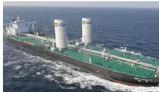
Wind-assisted propulsion system design as a whole with the hull
